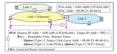
Figure 2: *Prefix Discovery* by means of *Router Solicitations*
